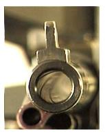
Inside the barrels of handguns and rifles are spiral impressions called rifling. The raised portions of the rifling are known as lands and the recessed portions are known as grooves. When a firearm is fired, these lands and grooves cut into the bullet, putting spin on it as it travels through the barrel of a firearm. Because bullets have an oblong shape, spin is necessary for accurate flight.
