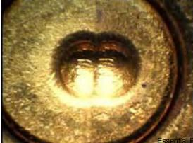
**Firing pin impressions** - When a firearm's trigger is pulled, the firing pin will move forward striking the primer cup located at the rear center of the cartridge.
