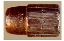
The impressions of lands and grooves are transferred to the bullet when it is fired.
