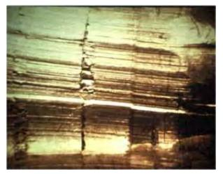
The second step involves using a comparison microscope to compare the test bullet to the bullet recovered from the victim or crime scene.
